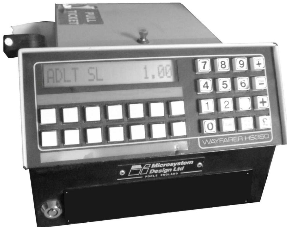
**A Wayfarer saver HS350 model, easily identified by the larger LCD screen, farestrip labels above the class buttons, and the HS350 logo located on the bottom right of the keypad.**
