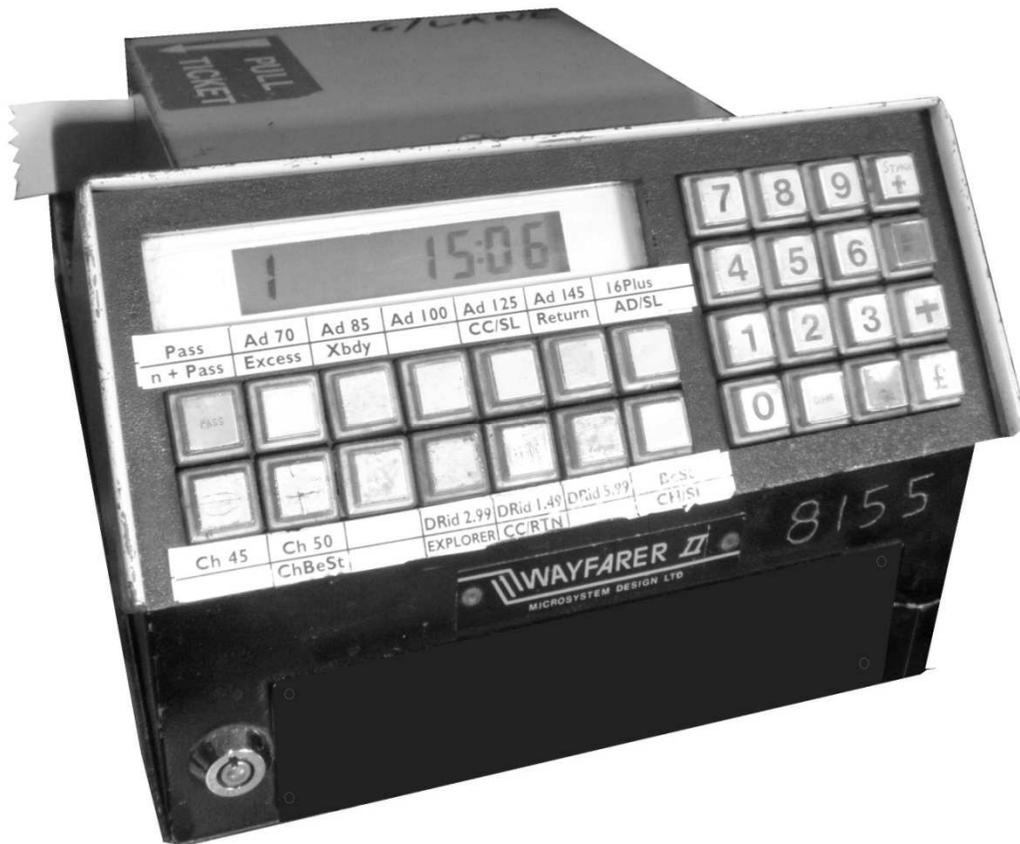
**A Wayfarer Saver 'Key Cap' machine. This can be identified by the smaller screen area, with a 'calculator' style display. Also the fare labels are usually either stickers above the buttons, or labels inside the button cap itself.**
